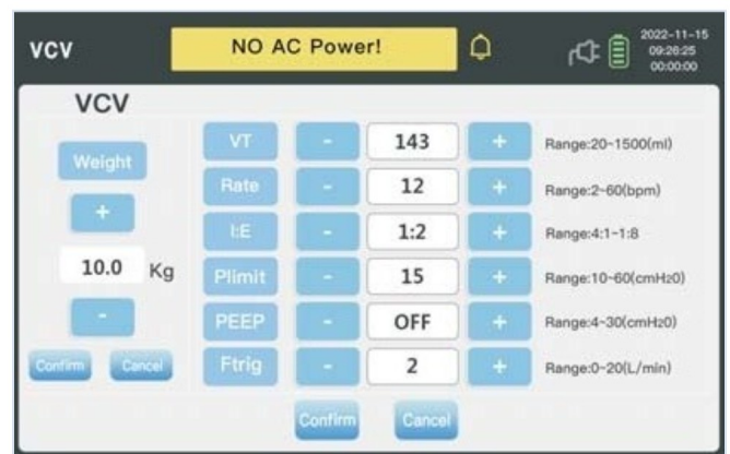
Enter the animal's weight to load suggested parameters, then fine-tune as needed
