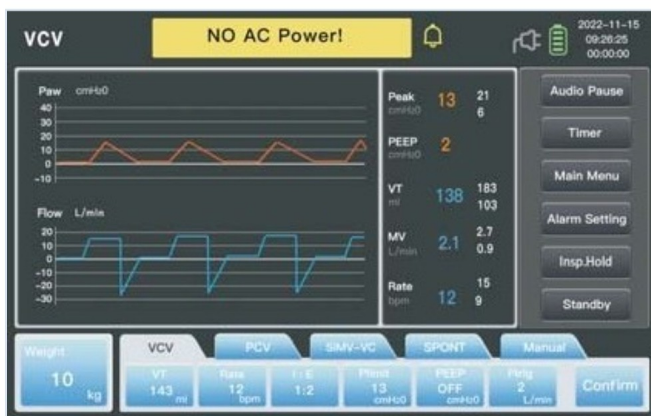
Main screen: real-time pressure and flow waveforms with peak, PEEP, VT, MV and rate
